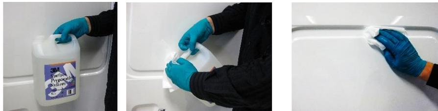
**Note:** Do not use isopropyl alcohol as this can affect the lifting resistance of the film in the recessed area. Other solvents than 3M™ Surface Preparation System may affect the expected lifting resistance performance of the film, too.
