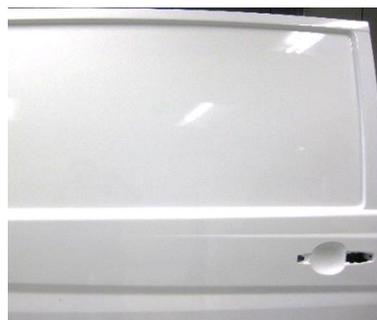
Position the film and apply it from the top and fix the edges of the contours.
