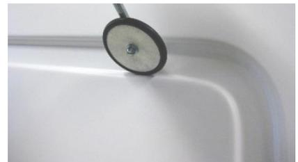
The hand-rollers (3M™ Deep Channel Rollers Small and Large) allow the film to be applied with uniform, continuous pressure and low friction.
