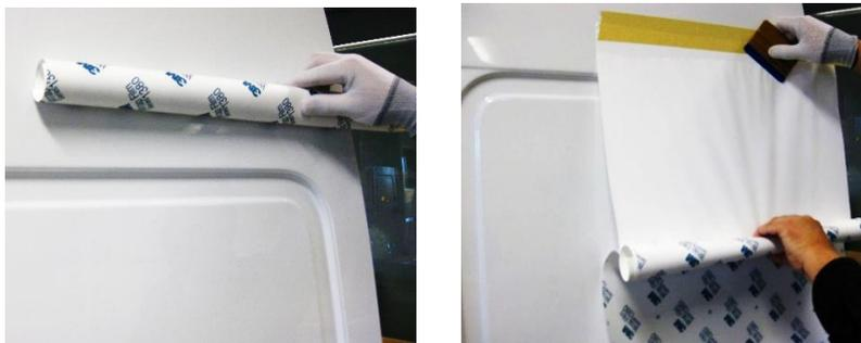
Films require high squeegee pressure to avoid air entrapment between film and substrate. Therefore the use of 3M™ PA-1 Gold Squeegee with thin and soft sleeve (e.g. microfibre) is recommended. Wetting of the sleeves helps to avoid scratches on the film surface during application.
