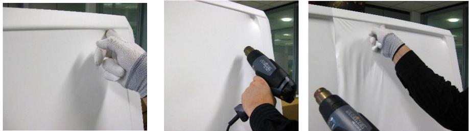
After the film is completely applied into the recess, apply the film on the remaining area within the recess.
