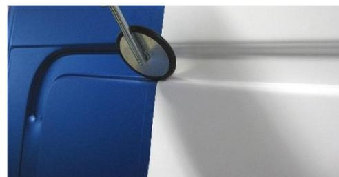
**CAUTION:** Re-heating of the film and repressing the film into the recesses and deep channels is a quality control measure to assure a good application without air bubbles.
