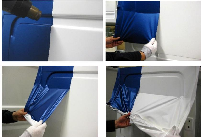
For fast heating of larger film areas the use of Infrared heater (2000 W, e.g. TERM 2000 CVH from company Burda Worldwide Technologies GmbH) is recommended.
